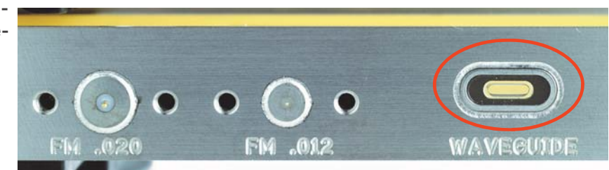
Waveguide window laser welded into aluminum housing
