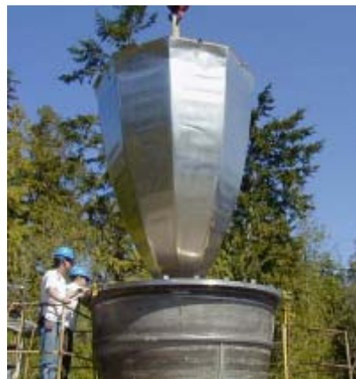
Space Shuttle Skin Before and After Explosive Forming
