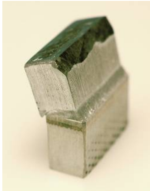
Aluminum/stainless steel hammer test
