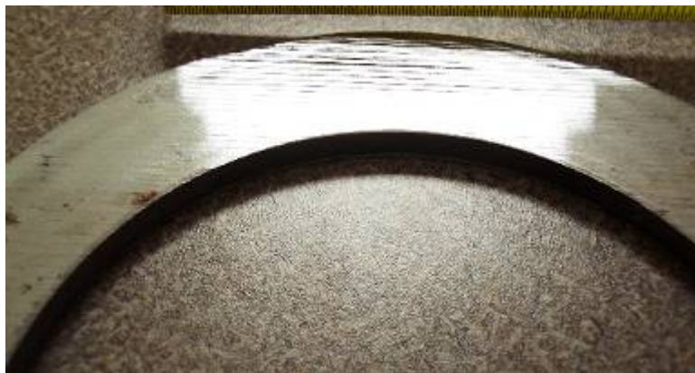
Tantalum on I.D. of steel pipe
