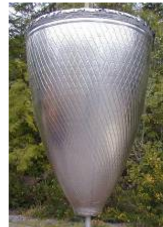
Space Shuttle Skin Before and After Explosive Forming
