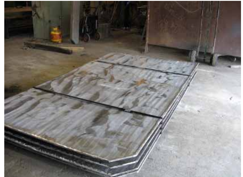
Plates after flattening
