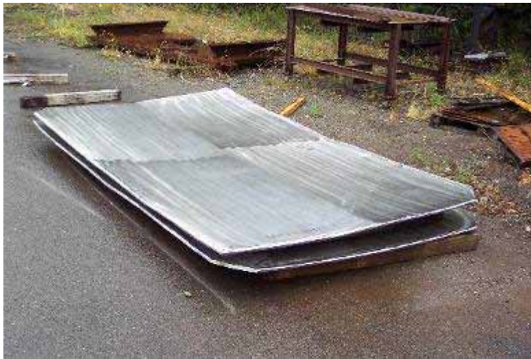
Ni/Inconel plates before flattening
